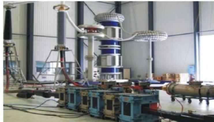
230kV cable and accessories test circuit
