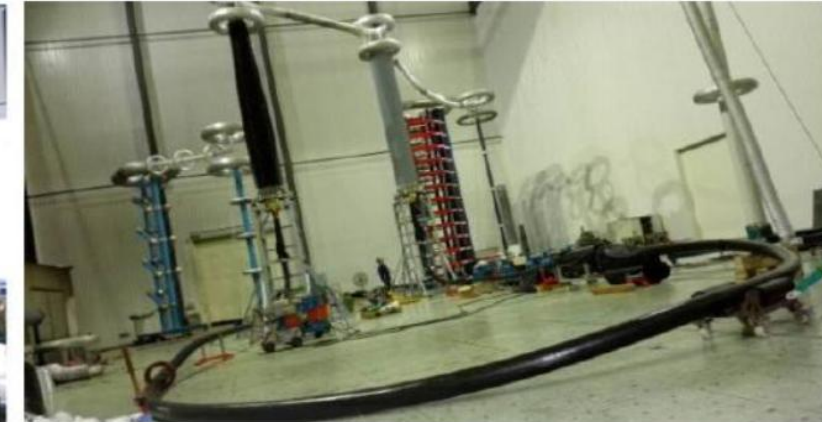
500kV cable and accessories test circuit
